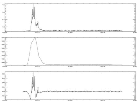
Figure 1: An example of the application of the algorithm for the automatic detection of the disturbances. The first time series is the original, the second is the smoothed and the third is the extracted. In this example the extracted time series has more than 10 instances where the counts exceed the  $4\sigma$  threshold, therefore this is a "disturbed" time series.
